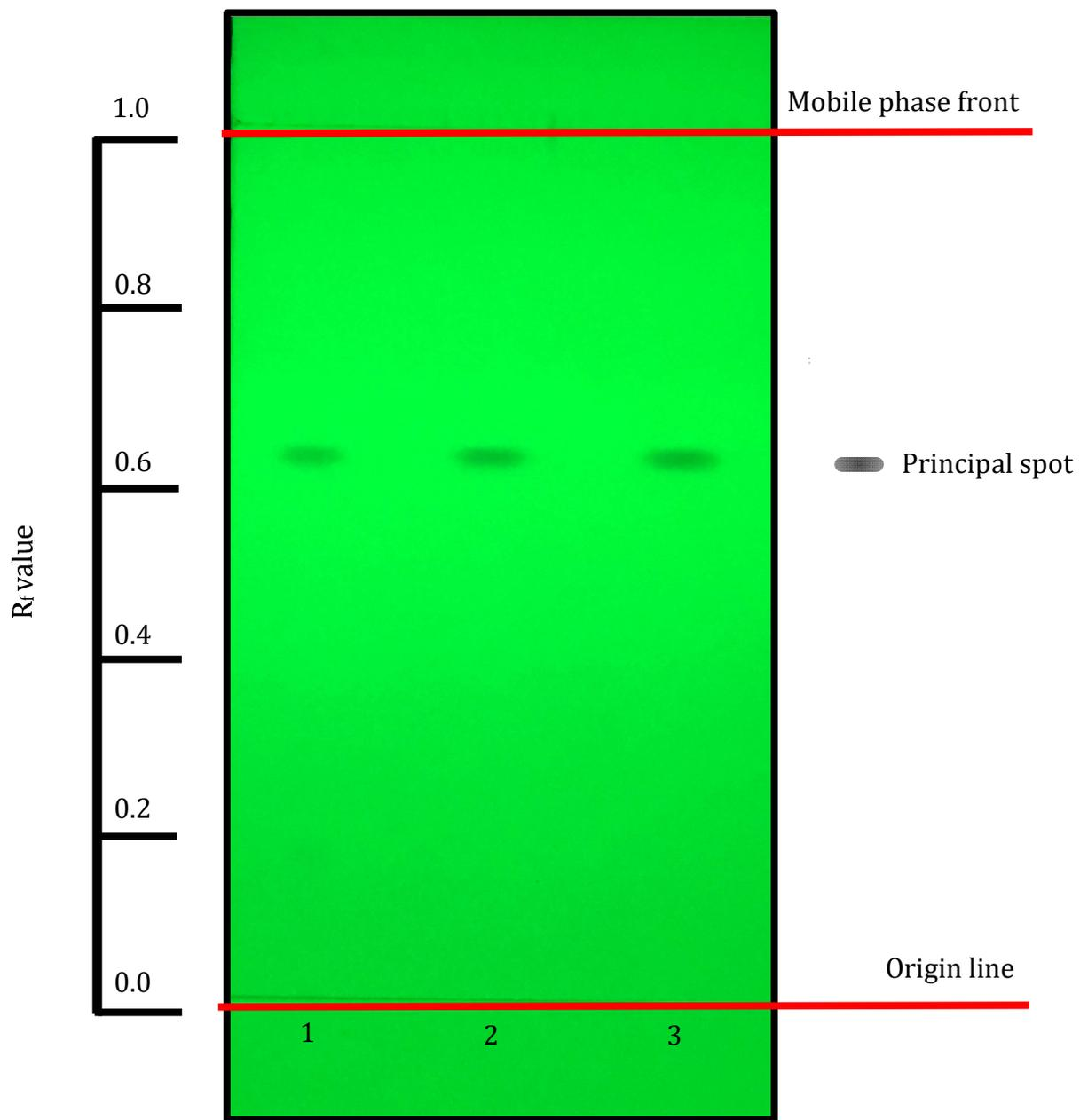
Plate observed under ultraviolet light at 254 nm
